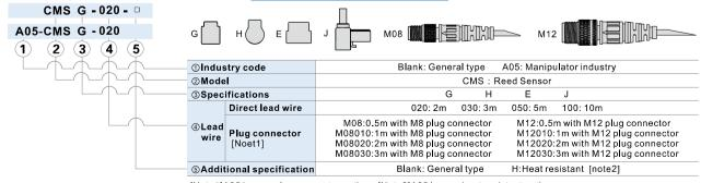
[Note1]A05 has no plug connector option. [Note2]A05 has no heat resistant option. Add:The sockets of M08 and M12 need additional order. Please check on page371.
