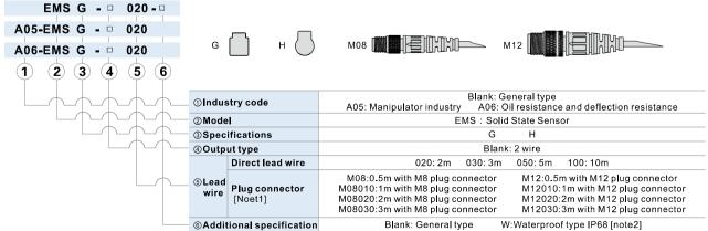
[Note1]A05 and A06 have no plug connector option. [Note2]A05 and A06 don't have a-w Waterproof option. Standard A06 model has a waterproof function. Add:The sockets of M08 and M12 need additional order. Please check on page 371.
