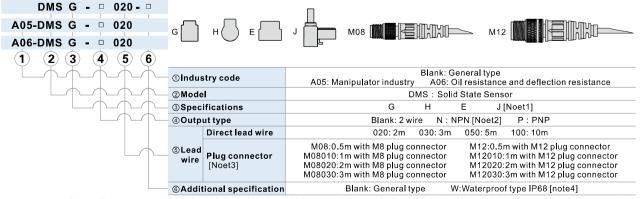
[Note1]Type J is not available for A06. [Note2]A05 and A06 have no NPN and PNP option. [Note3]A05 and A06 have no plug connector option. [Note4]A05, J type and M08, M12 don't have a-w Waterproof option. Standard A06 model already has a waterproof function. Add: The sockets of M08 and M12 need additional order. Please check on page 371.
